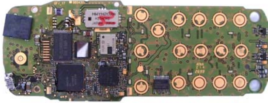
Figure 2: Stripped down view of the internal components and the several radio chips of a Nokia handset. (Wikipedia)
