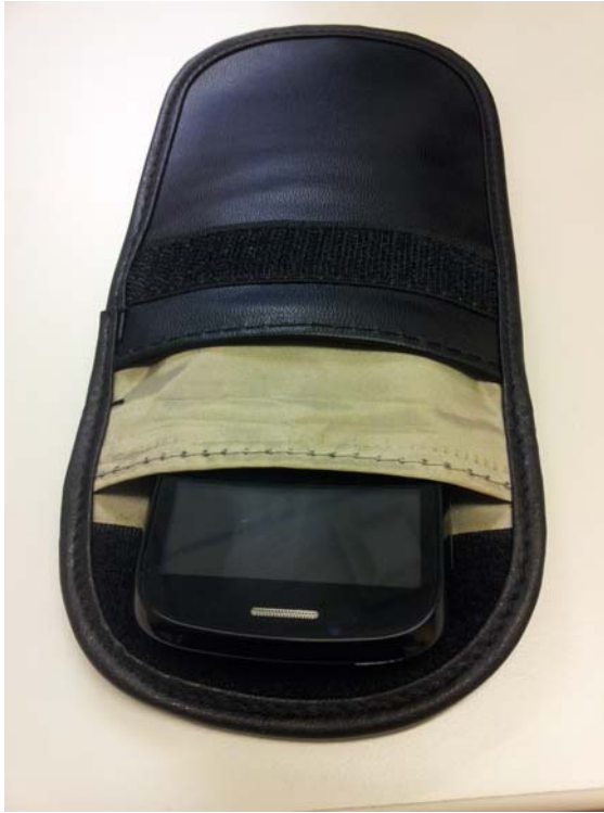
Figure 5: Signal blocking pouch with the Huawei Ideos partly immersed inside. The titanium coloured lining is the conductive mesh that makes up the Faraday cage when the pouch is sealed.
